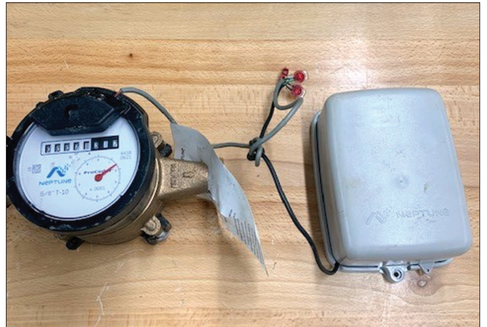
One of the Town of New Glasgow's new water meters with the R900 box that transmits the readings.
