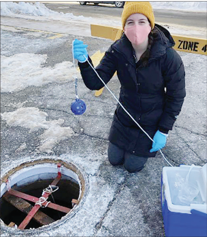
Genevieve Erjavec, a research assistant at the Dalhousie Centre for Water Resources Studies lab, deploys a COVID-19 Sewer Cage device at municipal manhole location for COVID-19 surveillance in wastewater.
